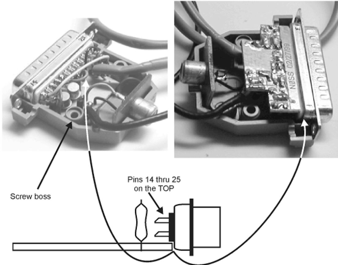
**Note:** The PC Board does NOT fit between the DB-25 pins, but just below the edge of the plastic insulator of the DB-25 connector. It will be held in place by the two screw bosses in the shell of the connector once the shell has been fitted to the connector.
